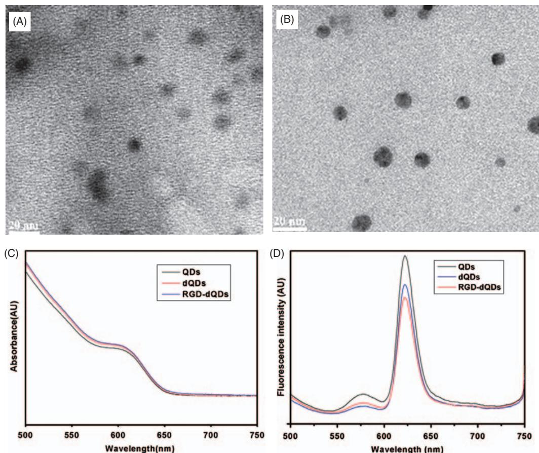
**Fig. 1.** Characterization of QDs, dQDs, and RGD-dQDs. (A) HR-TEM images of QDs. (B) HR-TEM images of RGD-dQDs. (C) and (D) UV-vis absorbance spectra and Photoluminescence spectra of QDs, dQDs, and RGD-dQDs.
